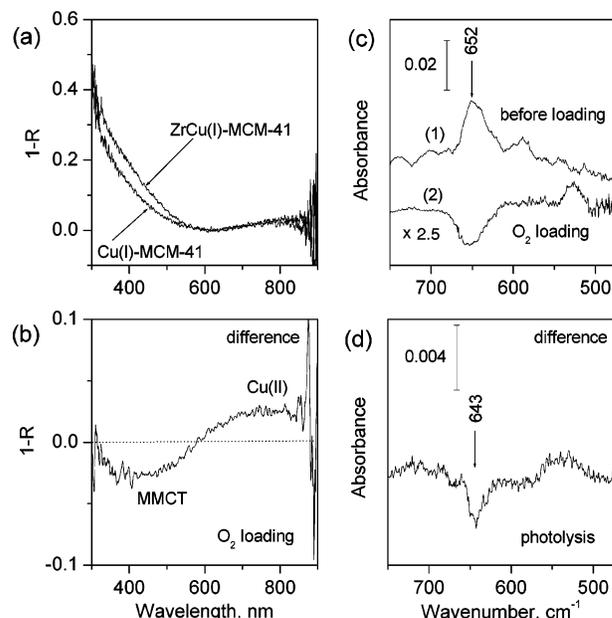
**Figure 1.** (a) UV-vis DRS of ZrCu(I)-MCM-41 and Cu(I)-MCM-41. (b) Difference DRS spectra recorded after and before exposure of ZrCu(I)-MCM-41 to O<sub>2</sub> gas (1 atm) at room temperature for 8 h. (c) FT-IR spectrum of ZrCu(I)-MCM-41 (referenced against neat MCM-41). (c2) Difference FT-IR upon exposure to 1 atm of O<sub>2</sub> gas for 24 h in the dark. (d) Difference FT-IR spectra after photolysis (355 nm, 165 mW cm<sup>-2</sup>, 2.5 h) of the CO<sub>2</sub>-loaded (1 atm) ZrCu(I)-MCM-41.
